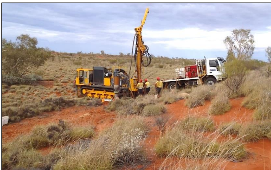
Figure 6.14: RC drilling at the Webb tenements – a total of 83 drillholes have been completed, with drillhole spoils (top image) being analysed for KIM and diamond content
